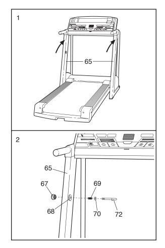
Press the Lock Knob Sleeve (68) into the left Upright (65). If necessary, use a rubber mallet to tap the Lock Knob Sleeve into the Upright.
